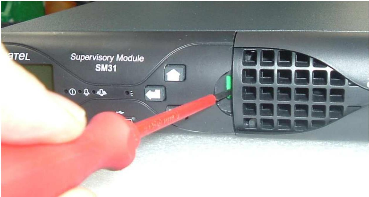
**Fig 4.** For removal, unlock SM3x by lifting green locking tab.
